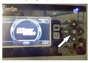
2. Press and hold the ESC (Escape) button to enter the screen.
