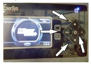
4. Navigate to "Password" then press the Enter/Power button. Enter the password 0 0 9 9 then Enter.
