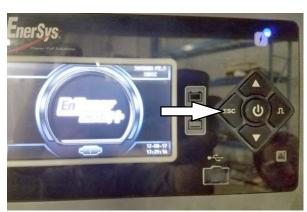
3. Press the four outer buttons as needed to navigate through screens in the following steps.
